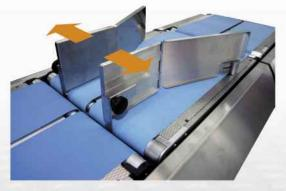
Automatic adjustment of alignment station.
