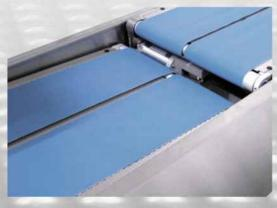
Labelling conveyor with lowering device for long packages, user-friendly with quick changeover.
